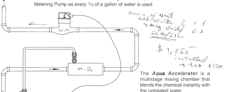
The **Aquadose** Chemical Metering Pump injects a precise amount of chemical under high pressure into the turbulent water stream created by the Aqua Accelerator.
